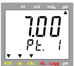
Place electrode and temperature probe (if any) in the neutral solution stirring gently. The measuring value is stable as soon as the display stops blinking and the 'ok'-arrow is
