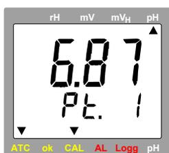
**DIN-series** (values at 25 °C: 1.68pH(A), 4.01pH(C), 6.87pH(D), 9.18pH(F), 12.45pH(G))
