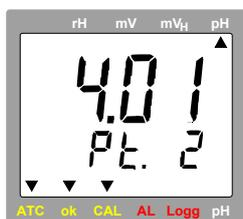
Place electrode and temperature probe (if any) in the buffer solution you want to use for the next calibration point (e.g. 4.01pH for the Standard series).
