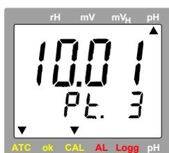
Place electrode and temperature probe (if any) in the buffer solution you want to use for the third calibration point (e.g. 10.01pH for the Standard series).
