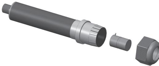
Fit the sensing element gently into the sensor. The correct position is indicated by a groove. Mind that you do not bend the connecting pins. Check the sealing ring and screw the screwcap on.
